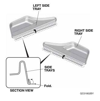
5. Place the left and right side trays in the both sides of the trunk. Insert the folded ends of the side trays into the gap as shown.
